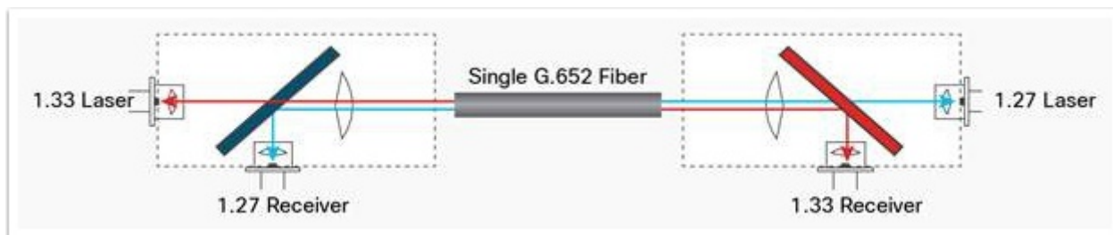
Figure 2. Bidirectional transmission of a single strand of SMF
